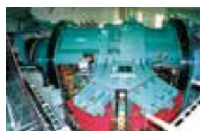
Rotating gantry (Height 10m, weight over 200t)
